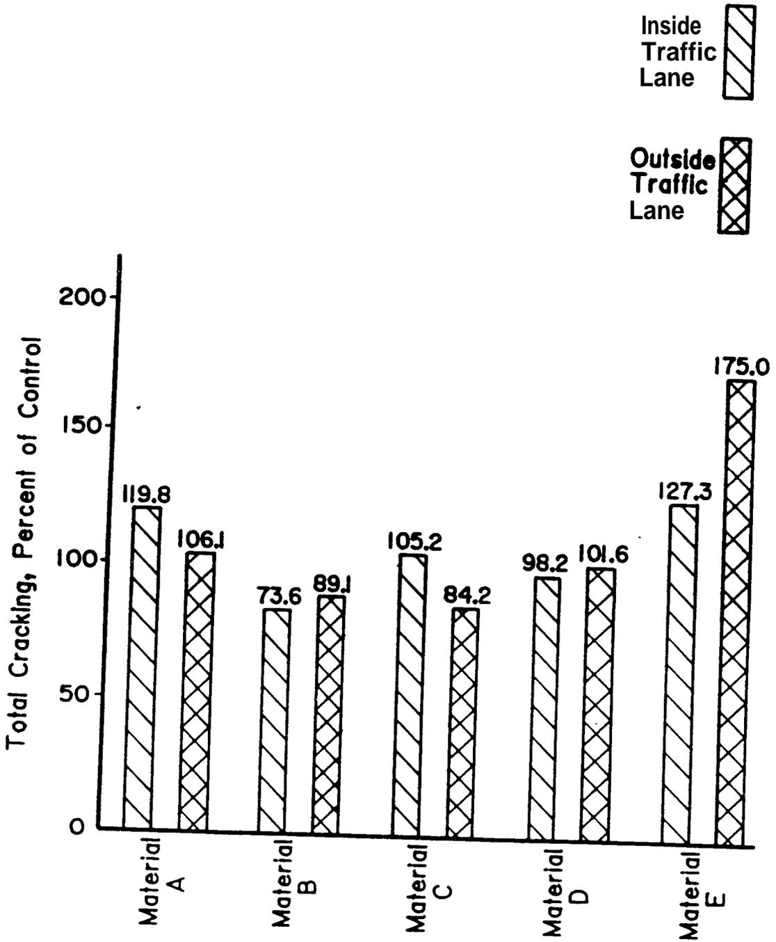
Figure 4. Relationship Between Material Type and Total Cracking
