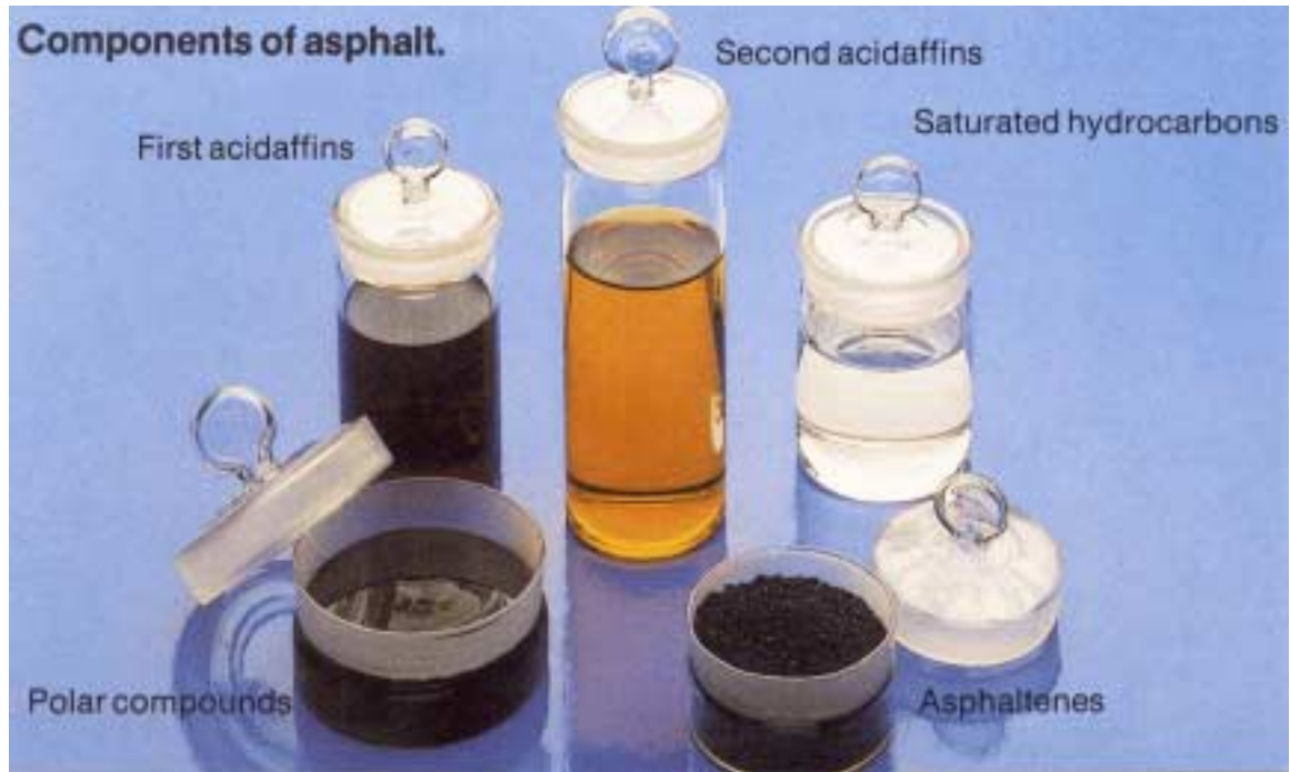
Figure 1. Asphalt Binder Fractions, Asphaltenes and Maltenes.
